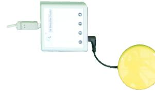
Open Notepad, or other text editor, and press the button. This is identical to pressing a key on a standard keyboard. The letter assigned to this button should be typed. If nothing appears follow the troubleshooting procedure.
