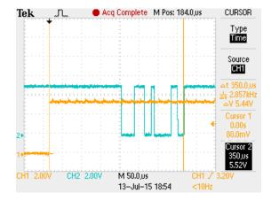
Typical time for 50 TTL outputs or event marking pairs (on|off) measured using our configuration and latency validation software for Microsoft Windows (Win 7 64 SP1, USB 2)
