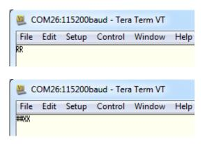
Once connected you will need to initialise it by sending the Module two RR bytes which resets the serial port and clears all TTL Output Lines.
