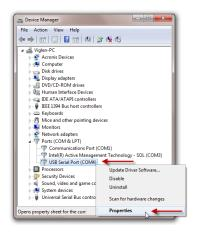
Right click on the USB Serial Port where the BBTK USB TTL Module was installed. Then click on Properties.
