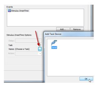
Next click on the more button ... and select the Serial port object so that you can write to the USB TTL Module.
