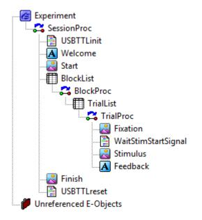
In this example as before there are two pieces of InLineScript that reset the USB TTL Module and are called at the start and end of the experiment.
