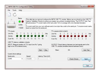
If you have chosen the correct COM port and the USB TTL Module is attached then the Status LED will change from red to green as shown and the interface will be unlocked.
