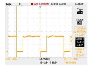
Typical time to send a TTL output or event mark (orange) from a two byte hex code from the PC (blue)
