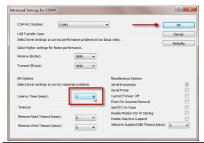
Under Advanced Setting for COMx you should select a Latency Timer (msec) of 1mS using the drop down box.
