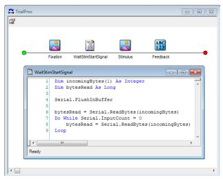
In this example execution will pause at the InLine code as the Do While Loop waits for any input change signalled by two incoming serial bytes from the USB TTL Module.
