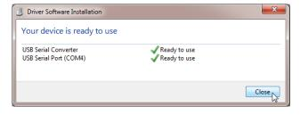
As part of the final step the Module will be assigned a USB Serial Port COM number. In this example, COM4. This is the serial port you would connect to the USB TTL Module through in order to event mark.
