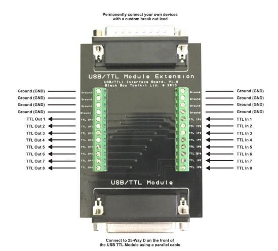
Using the Module to event mark is simple. Once installed all you need do is open the linked serial port and send a two byte hexadecimal string. For example to event mark on TTL Output Line 1, open the serial port and send the hex bytes 01. To stop send 00.
