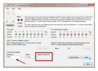
Under Current driver settings the COM port with the USB TTL Module attached should be automatically selected (red arrow).
