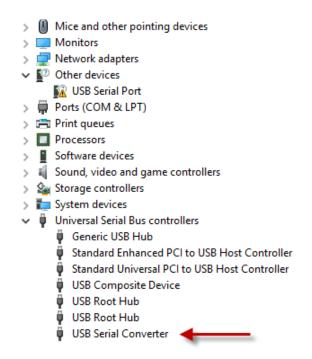
Once the drivers for the FTDI interface chip the USB TTL Module uses have been installed you will see a new entry for a USB Serial Converter under Universal Serial Bus controllers.
