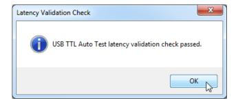
The test will be flagged as being passed if the mean latency is consistently under 1mS.
