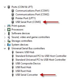
After installing the drivers you should see a new USB Serial Port, COM3 in this example and also an entry for a USB Serial Converter.
