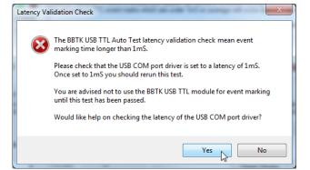
If the mean event marking time is longer than 1mS you will be warned and advised to check the COM Port Driver latency and offered help on how to do this.
