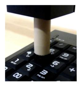
Once you have established your specific RKA start-up latency you are ready to test your response device. When you construct Stimulus-Response sequences in DSCAR etc. remember to use the corrected RKA RT and duration, i.e. 285ms RT and 105ms duration in this example. Remember RTs recorded by your paradigm should equal 300ms and 100ms duration and not 285ms and 105ms.
