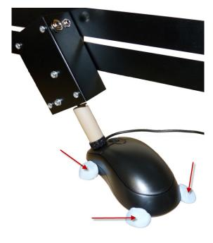
Anything which is used to temporally fix posters to walls should work well when rolled into a ball and compressed against your response device.
