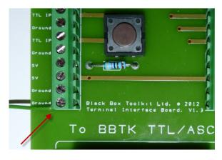
The other end of the Grounding Wire needs to be inserted into a grounding terminal on the Breakout Board. Here it has been terminated in the Ground bottom left of the Breakout Board.
