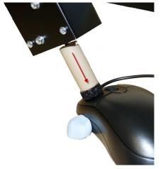
Note how the plunger and solenoid enclosure has been adjusted to an angle appropriate for reliably pressing the mouse button (red arrow).
