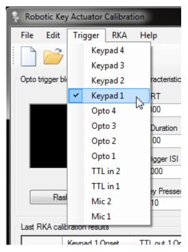
You can also change the trigger which signals to the RKA to make a response. In the example shown opposite the BBTK Keypad 1 button is used to trigger the RKA plunger.
