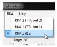
If you have more than one RKA, or would like to simultaneously generate a TTL signal on TTL Out 2, you can change output settings under the RKA menu.
