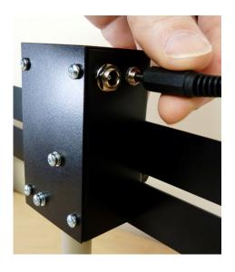
Plug the 3.5mm RKA TTL Trigger Lead jack into the 3.5mm socket on the solenoid enclosure.
