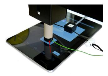
In the example shown opposite the RKA has been positioned above an on-screen button. An Opto-detector is positioned over a white marker block so that a RKA response is triggered when using DSCAR. The trigger block will need to switch from black to white when you wish to trigger the RKA.
