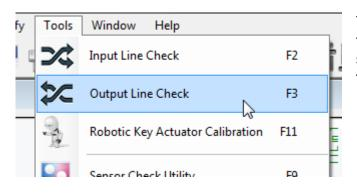
To test the RKA is working correctly start the Output Line Check utility in the PC software by pressing F3 or by selecting it from the Tools menu.
