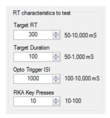
The RKA calibration routine has various settings which can be altered depending on your requirements.
