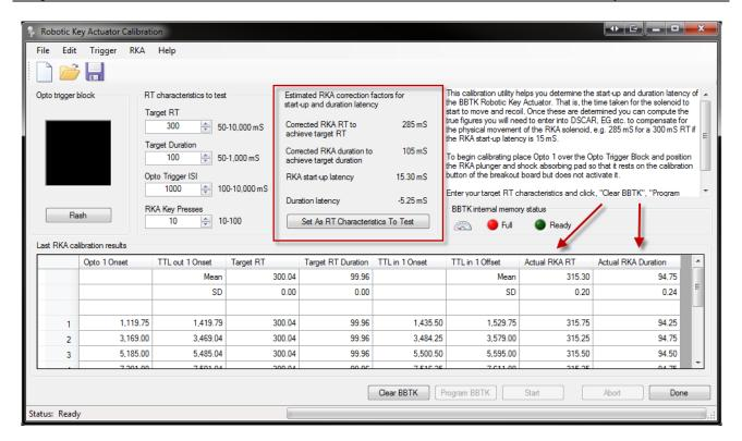
Details of the correction factors that need to be used are also shown in the middle frame (red box). In this case the RKA start-up latency was 15.30ms too long and the duration 5.25ms too short to achieve the target RT of 300ms with duration of 100ms.
