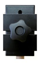
Loosen the thumb wheel to move the solenoid enclosure and plunger left and right across the gantry and vertically up and down. When you are happy tighten the thumb wheel.
