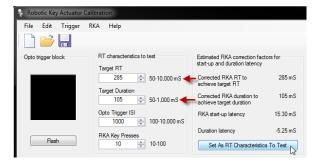
To verify the corrected figures are suitable you should rerun the calibration routine again after clicking on Set As RT Characteristics To Test. This will copy the corrected figures into the Target RT and Target Duration boxes (red arrows).
