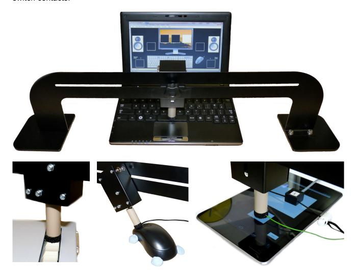
The RKA is a activated by sending a TTL output on TTL Out 1 in response to a stimulus trigger, e.g. a visual stimulus detected on one of the Opto-detectors. When activated it will press the key, or touch screen, for the duration you specify.
