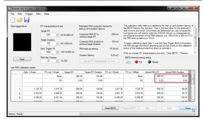
When the calibration run finishes the Actual RKA RT and Actual RKA duration columns should match your original target RT and duration, i.e. 300ms and 100ms respectively (red box). You are unlikely to achieve exact targets as the RKA is a mechanical device and is not comparable to using a more precise TTL to TTL signal.
