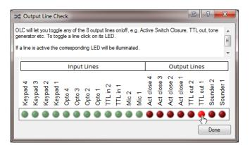
Each time you click on the TTL Out 1 LED the RKA should activate and stay active until you click on the LED again. That is, it should press and then release.
