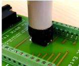
To begin position the RKA plunger centrally above the Calibration Button on the Breakout Board.
