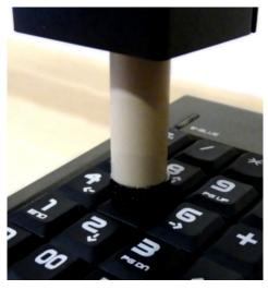
The foam should rest on but not activate the key. You can pull the plunger down manually to test fit and to make sure the key is activated when pressed. The aim is to replicate the fit when you calibrated the RKA using its calibration button.
